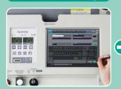
Input patient information with the touch-screen panel. By selecting the exposure menu on the CR Console, exposure factor (kV, mA) will be set on the x-ray operation panel.
